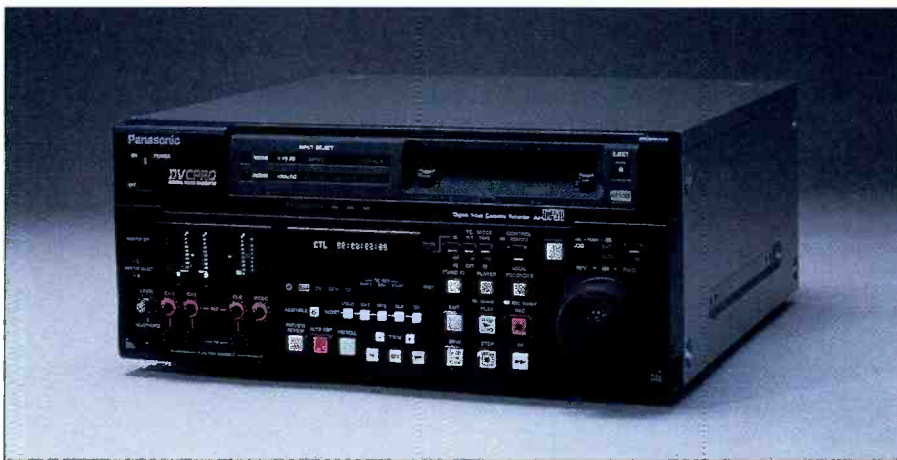
The AJ-D750 digital studio VTR provides complete versatility for editing applications. Tapes can be dubbed into the unit's HDD at four times speed, thereby shortening editing time.
